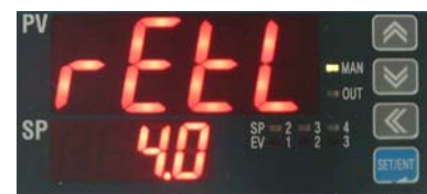
Figure 3: The SP value when 4 mA will be output by retransmitting outputs
