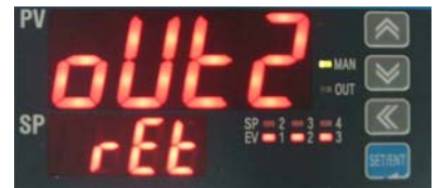
Figure 6: Setting an analog output to be a 4-20 mA retransmitting output
