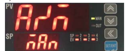
Figure 7: Setting the Auto/Manual parameter for manual control output operation
