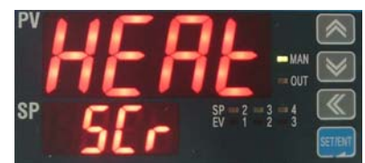
Figure 9: Setting the control output to transmit a 4-20 mA signal
